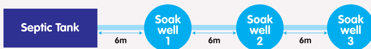
Fig. 8: Simple diagram of series soak well
